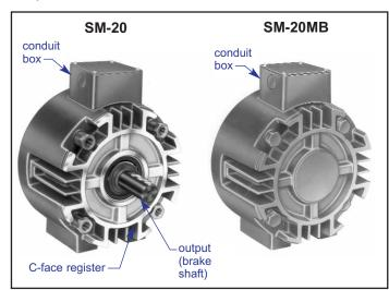
The Stearns Super-Mod series incorporates a Stearns gap feature that provides consistent de-energized armature-tofriction-face air gap. While the Stearns gap feature is desirable in most applications, the SM Series product can be ordered without auto gap for very soft starts and/or stops achieved through under voltage energization of the coil.
