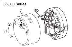
Remove housing nuts (15) by unscrewing from housing studs (150). Remove housing (7) by pulling back.
