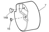
Remove manual release knob (148), housing nuts (15) and housing (7) by pulling back.
