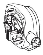
Series 65,000 brakes use four bolts (15S), threaded into endplate and four lock washers (15W). Remove all and pull back on housing (7) to free it. **Note:** Some older design Series 65,300 brakes used the same bolt arrangement as Series 65,000.
