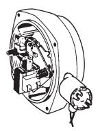
Series 65,300 brakes use four through-bolts (15S), four flat washers (15U), four lock washers (15W) and four hex nuts (15N). Remove all and pull back on housing (7) to free it.
