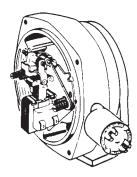
Series 65,000 brakes use four through-bolts (15S) threaded into endplate, and four lock washers (15W). Remove all and pull back on housing to free it.
